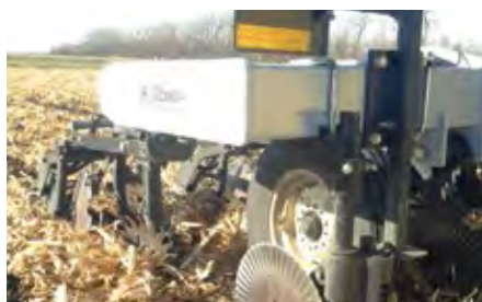
Strip tillage in corn residue provides soil incorporation on 30-inch rows where the seed will be placed the following year.
