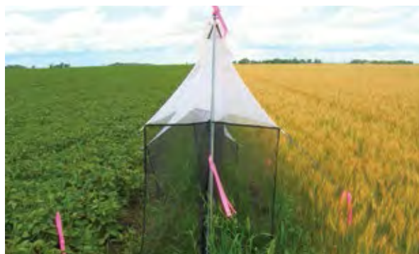
Fig. 2. Bi-directional Malaise trap used to monitor movement of predators between neighbouring fields. Insects are captured in separate collecting jars in each side of the trap.
