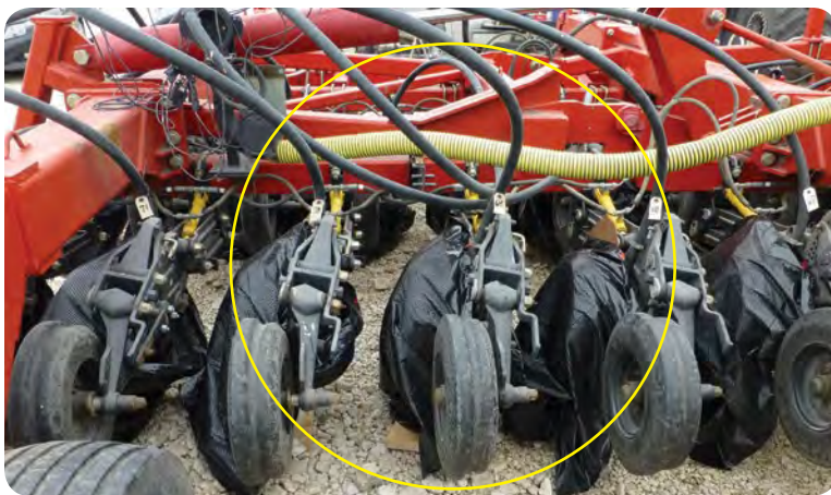
Bags were placed around each opener to collect product during each repetition.
