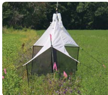
Figure 2. Bi-directional Malaise trap between soybeans and alfalfa to measure the movement of natural enemies between each crop. Insects are collected in jars on either side of the trap.
